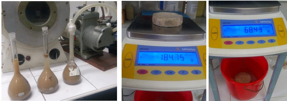
Figure 3.23 Pycnometer method to detect particle density (at left) and oven-dried weight (at middle) and Archimedes weights of the samples (at right) to find out their bulk densities.
