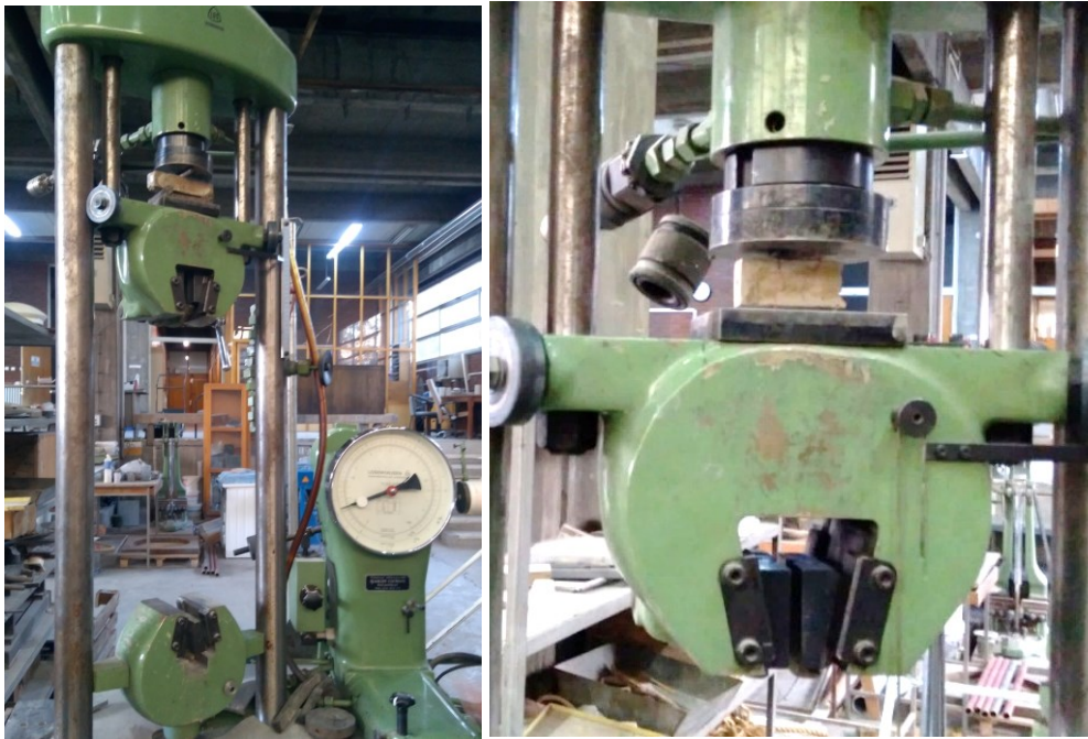
Figure 3.26 Flexural (at left) and compressive strength tests (at right) by the manual testing machine, LOS (Losenhausen, Maschinenbau AG Dusseldorf).
