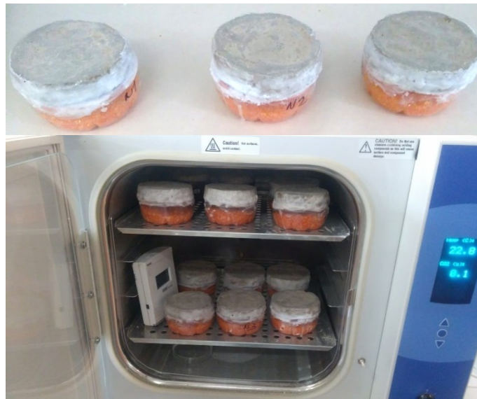
Figure 3.25 The samples kept in the test chamber in the dry cup method.
