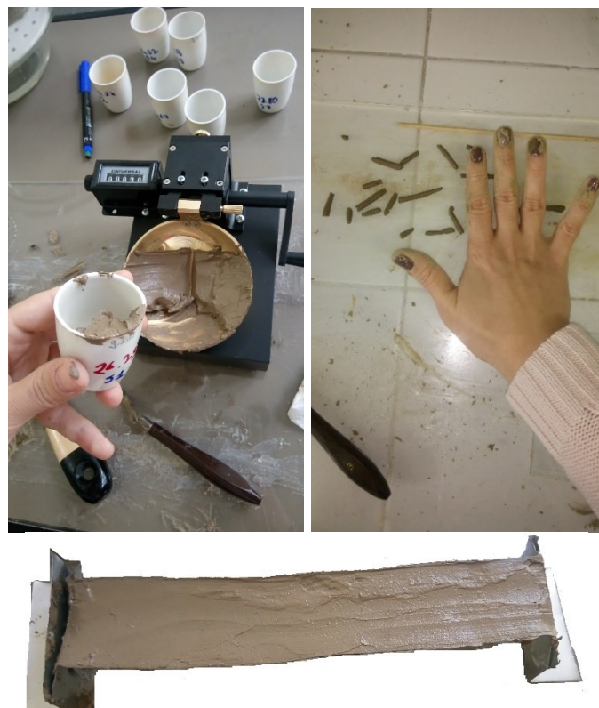
Figure 3.18 Liquid limit test performed by Casagrande apparatus (at top left) plastic limit test (at top right) linear shrinkage test (at the bottom).
