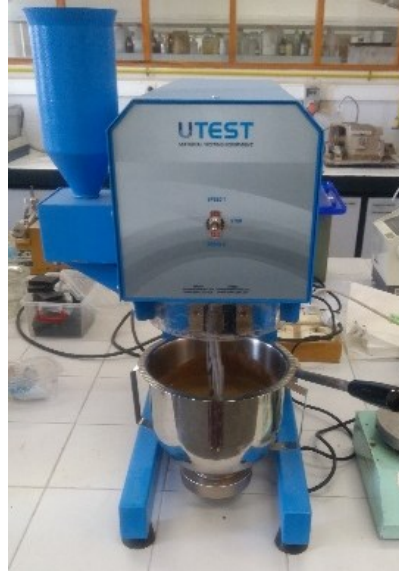
Figure 3.17 Mixing the soil sample in a higher amount with the laboratory mixer (Utest laboratory equipment).
