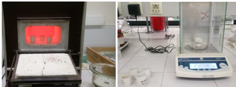
Figure 3.4 The soil samples heated at 105^\circ\text{C} , 550^\circ\text{C} and 950^\circ\text{C} , respectively, in the oven and weighed after each heating.
