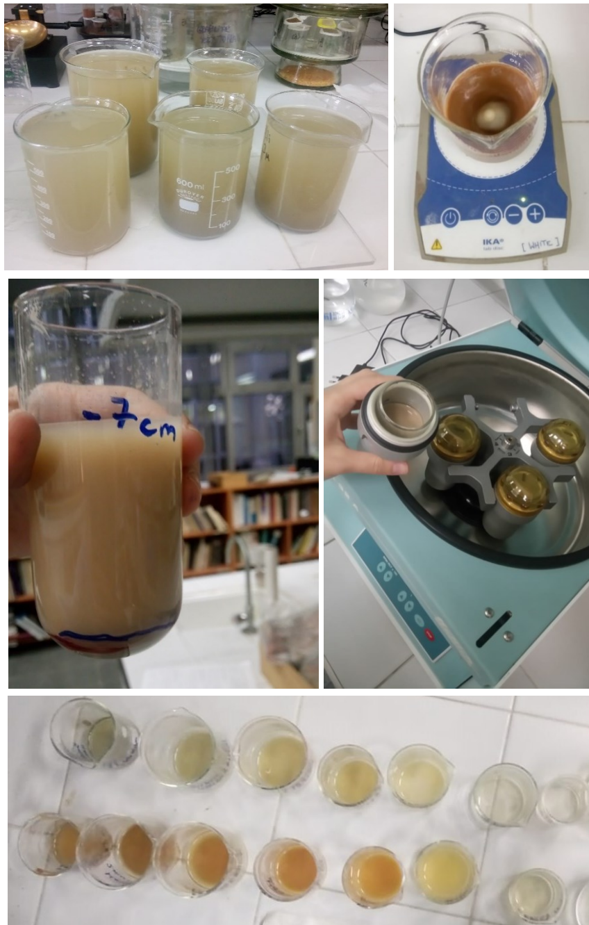
Figure 3.14 Determination of the particle size below 63 \mu\text{m} s by centrifugal sedimentation.
