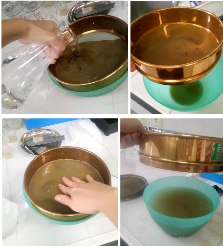
Figure 3.8 Steps of the wet-sieving to separate the silt-clay content from the sand and gravel.
