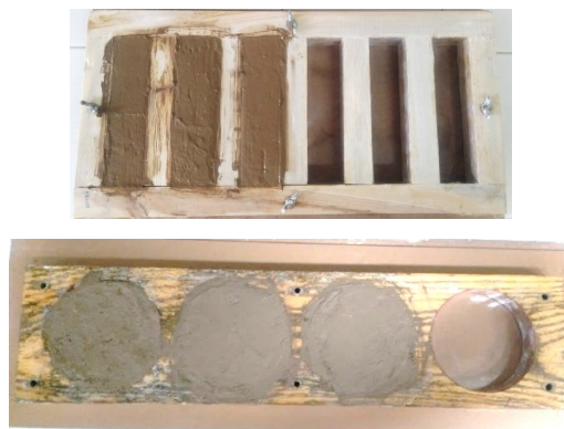
Figure 3.21 Moulded samples in 4x4x16 cm (at left) and in 10cm-diameter and 2.5 cm-height (at right).
