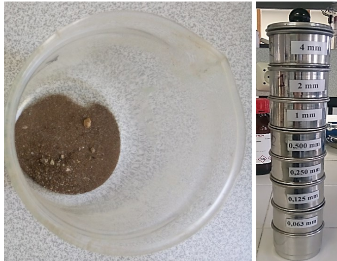
Figure 3.11 Determination of the particle size above 63 microns by dry-sieving.
