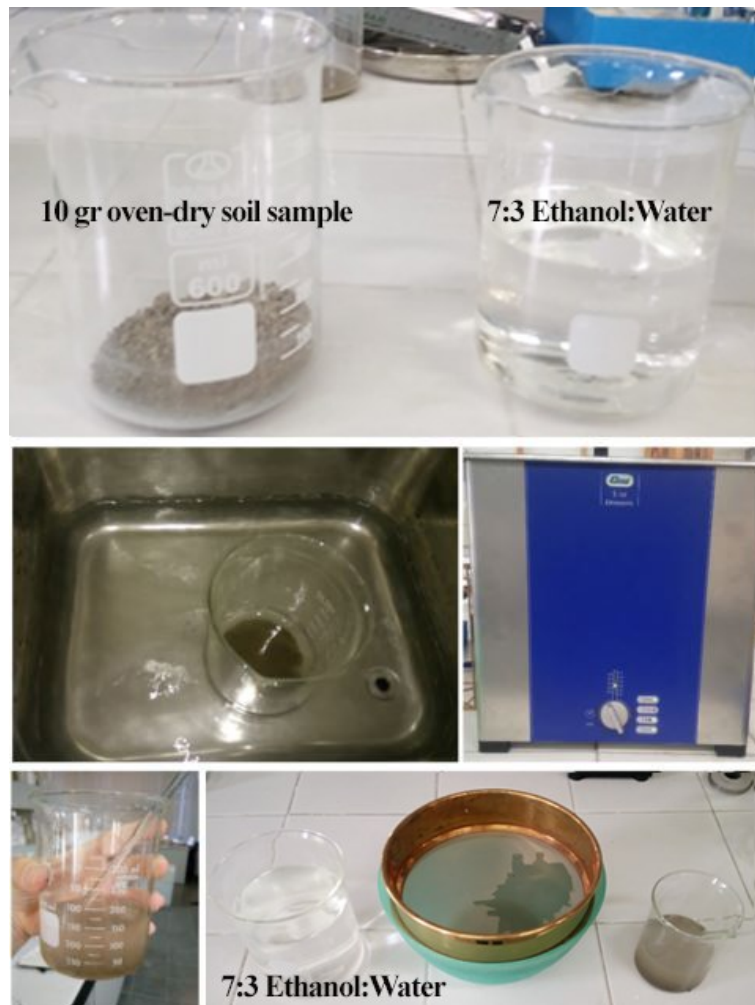
Figure 3.9 Steps of alternative method including sonication analyses (ultrasonic bath: Elmasonic S120 at 37 kHz, 200W) and wet-sieving to separate the silt-clay content from the sand and gravel.
