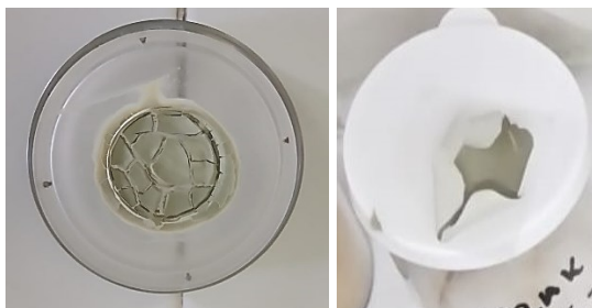
Figure 4.10 Excessive crack and shrinkage problems on the diluted sample of Eskişehir_Sazak.
